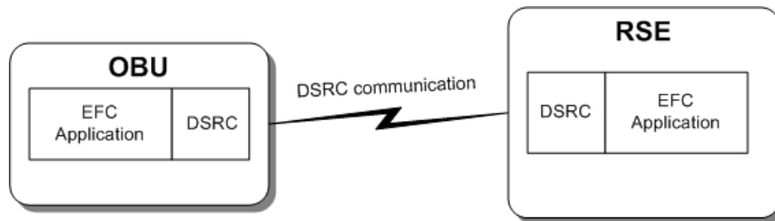
Figure 1: DSRC communication and EFC application
