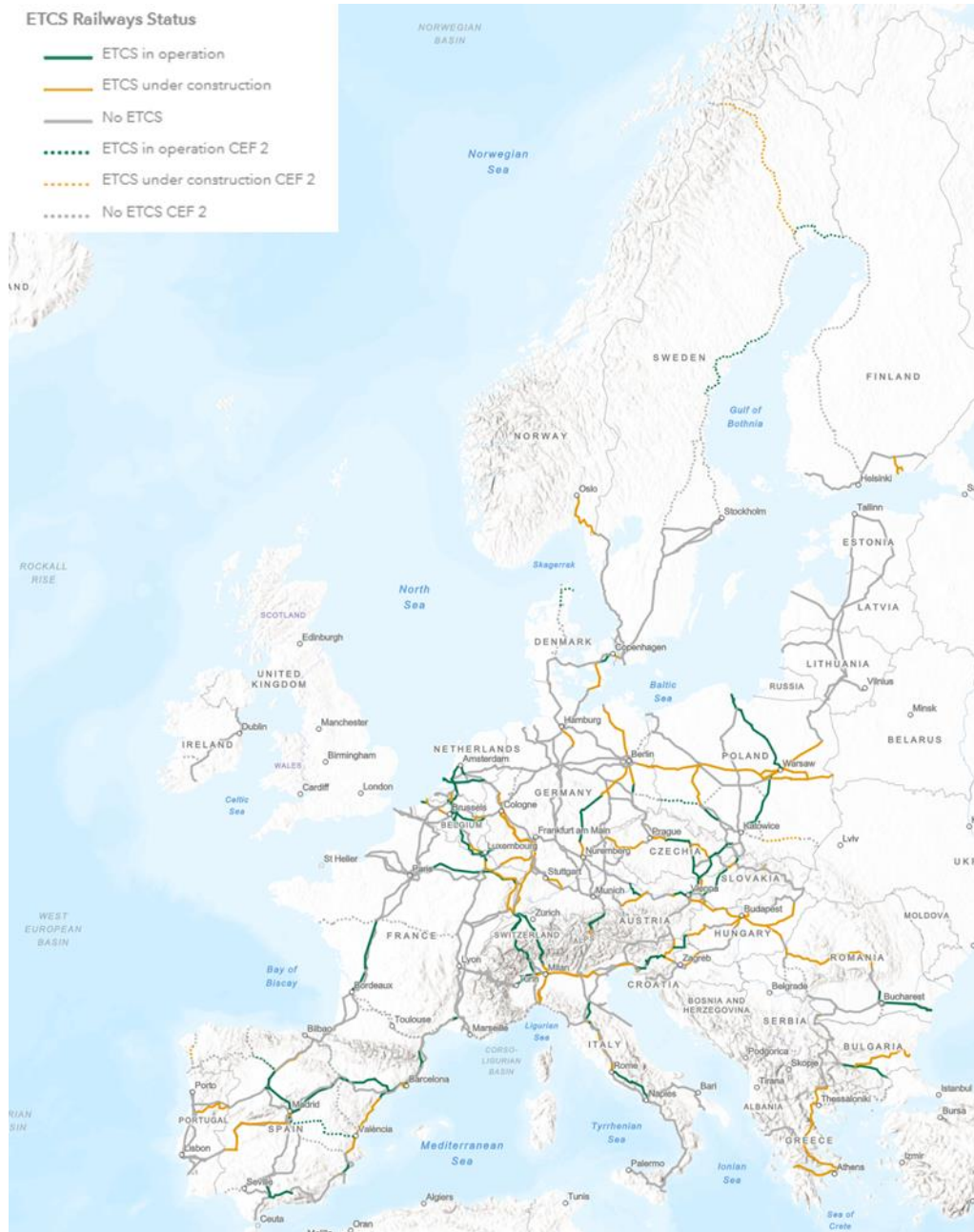
ETCS status: no ETCS, ETCS under construction & ETCS in operation (Source: DMT elaboration)
