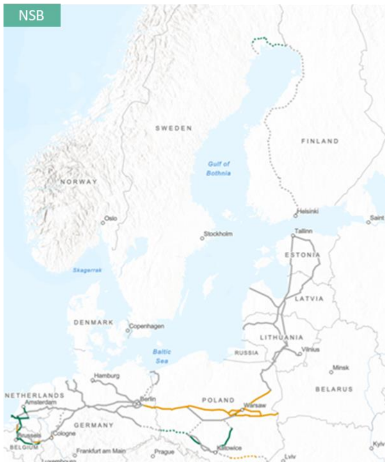
CNC NSB ETCS status: no ETCS, ETCS under construction & ETCS in operation (Source: DMT elaboration)
