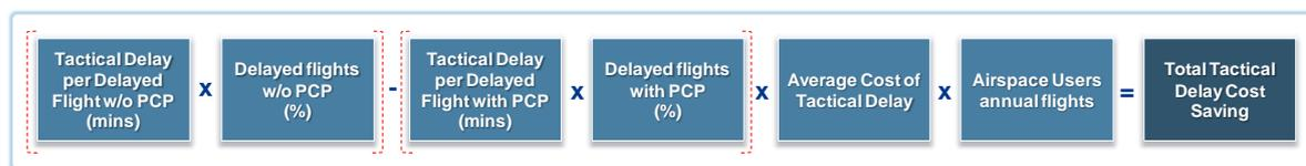
**Figure 48: Tactical Delay Cost Savings monetisation mechanism**
