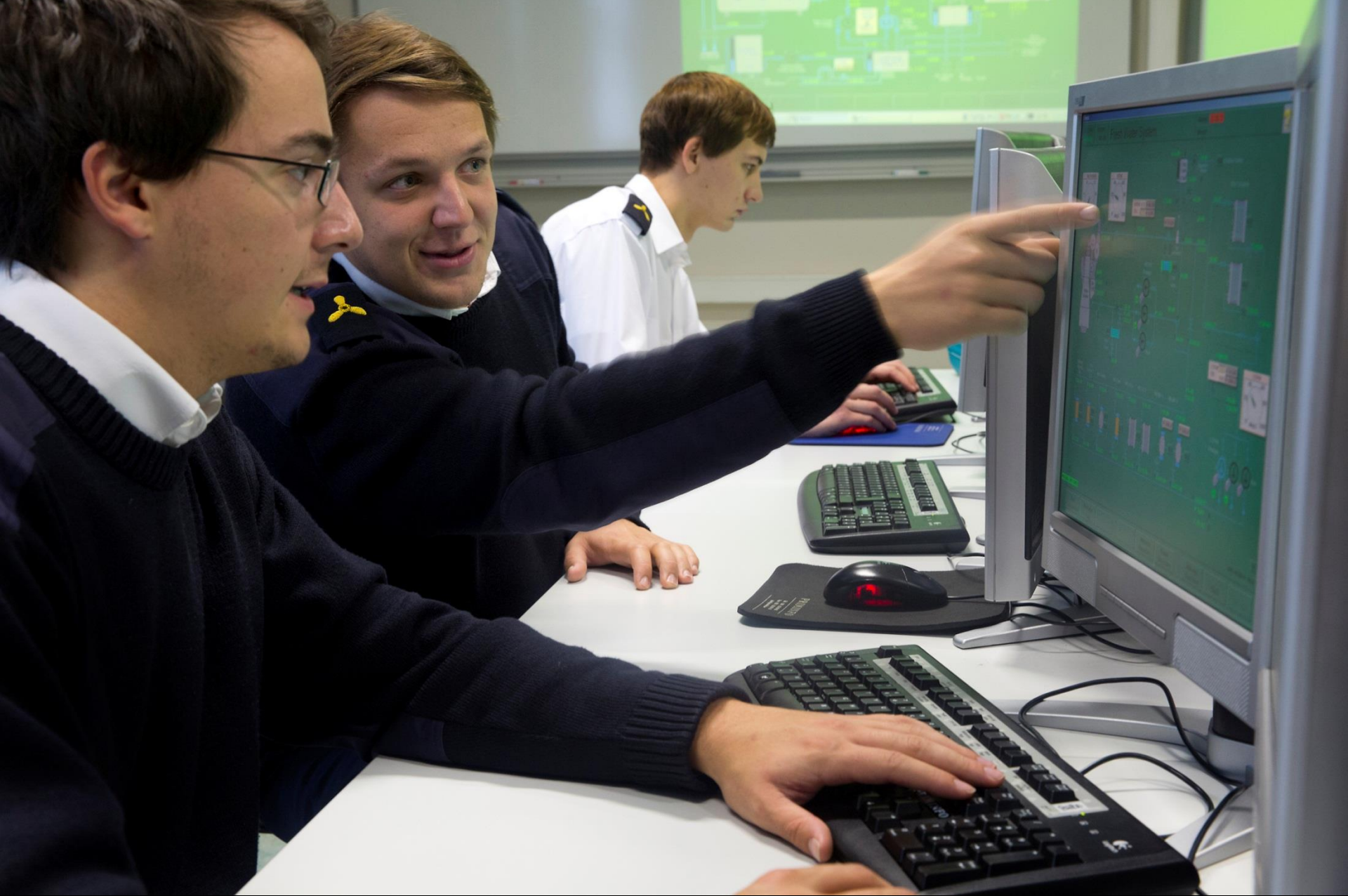
PPT (Propulsion Plant Training) simulates an engine room control centre.
