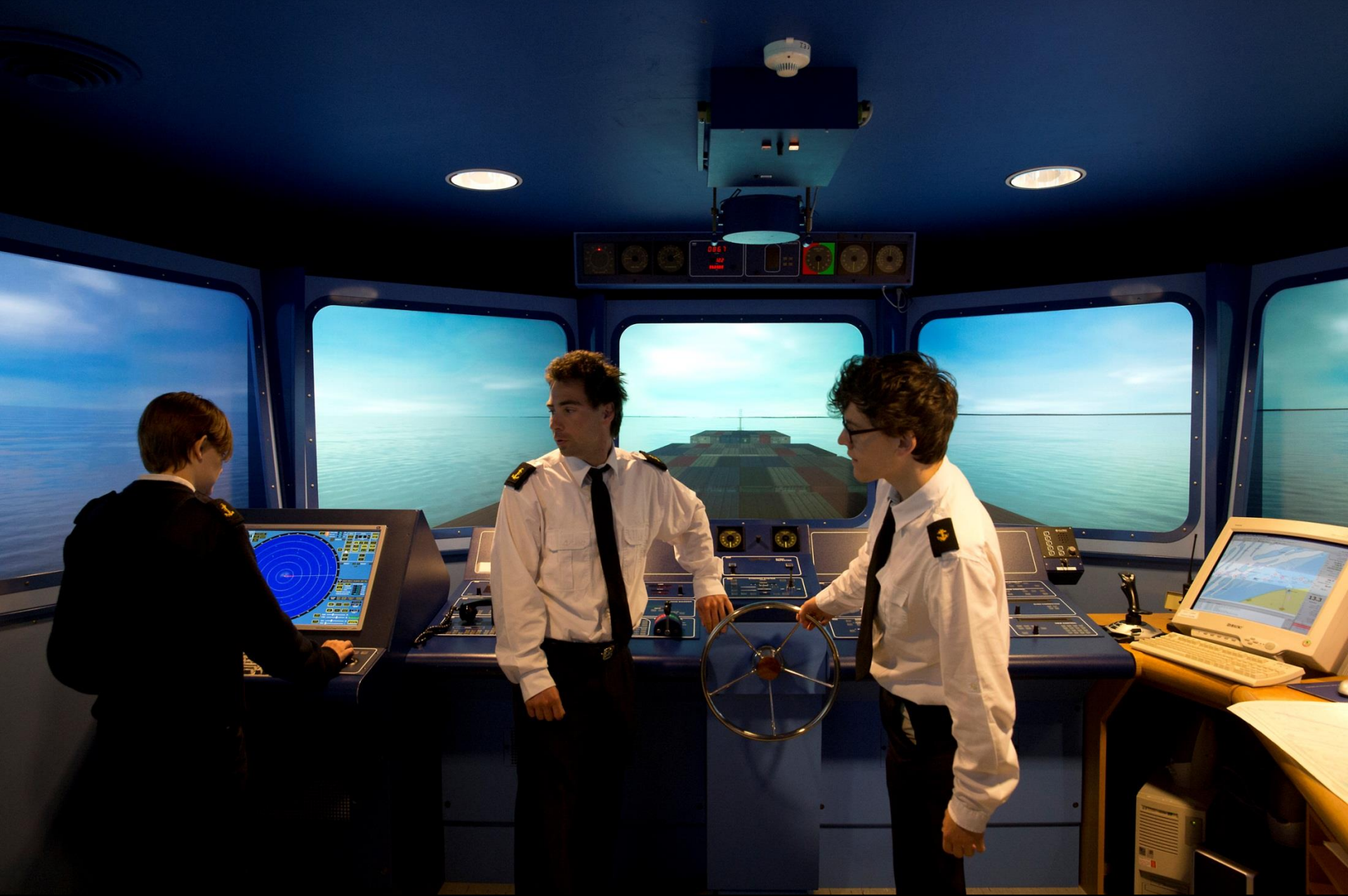
Full Mission Bridge Simulator to train radar and navigation techniques.
