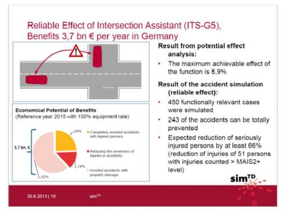
Figure 8 - Reliable effect of Intersection assistant (ITS-G5)
