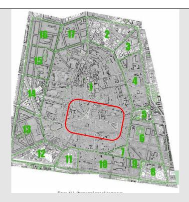
The scheme is based on the permit distribution concept and on the ground enforcement system that works by reading the number plates of all vehicles entering and leaving the city centre. If the vehicle entering the regulated zone takes less than a certain time to exit the regulated area, the system considers it as a 'passing-through' vehicle and the driver is fined.
