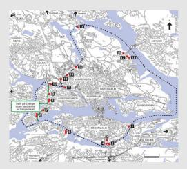
The system features 18 control points located at Stockholm city entrances and exits. Vehicles are automatically recorded by cameras capturing the number plates. Images of vehicles equipped with an electronic onboard unit (transponder) for direct debit payment are also identified in this way.
