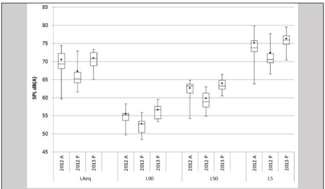
Figure III: Variation of the equivalent and percentile levels for the entire soundwalk over the years (Maffei et al., 2013a)
