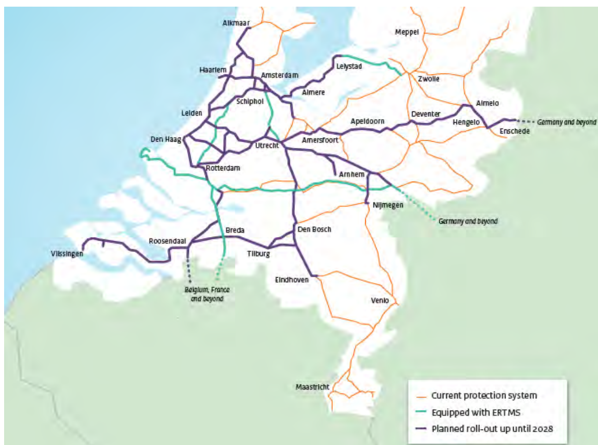
Figure 65: Introduction of Summary of already realised and previously agreed rollout of ERTMS to 2028
