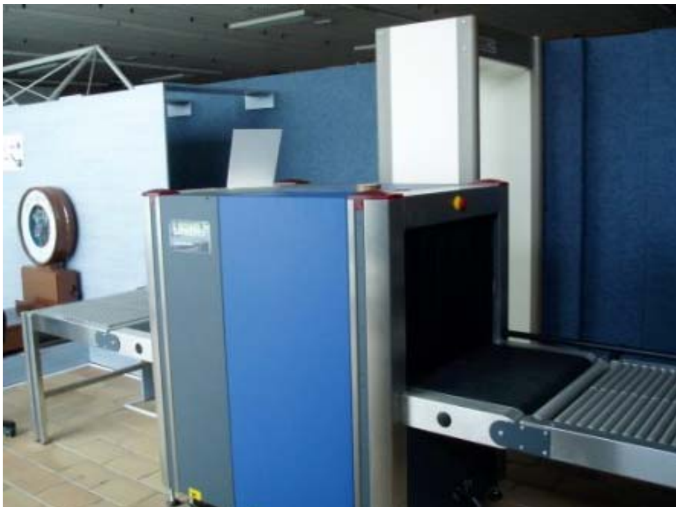
Baggage x-ray and metal detection machine.
