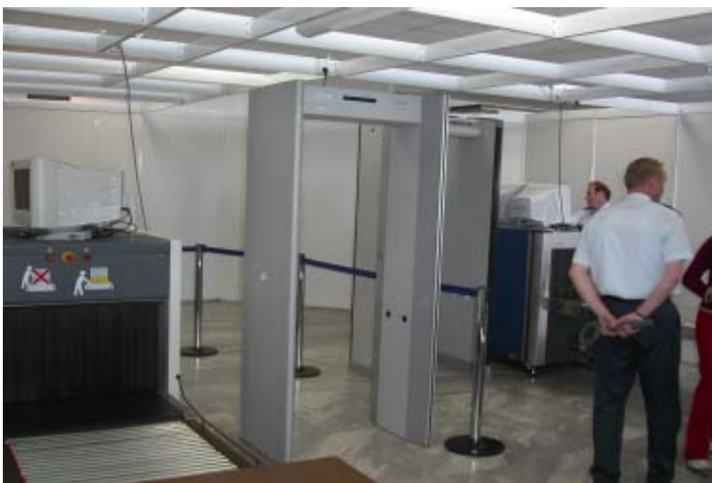
Passenger security check area with two x-ray machines and two metal detectors.
