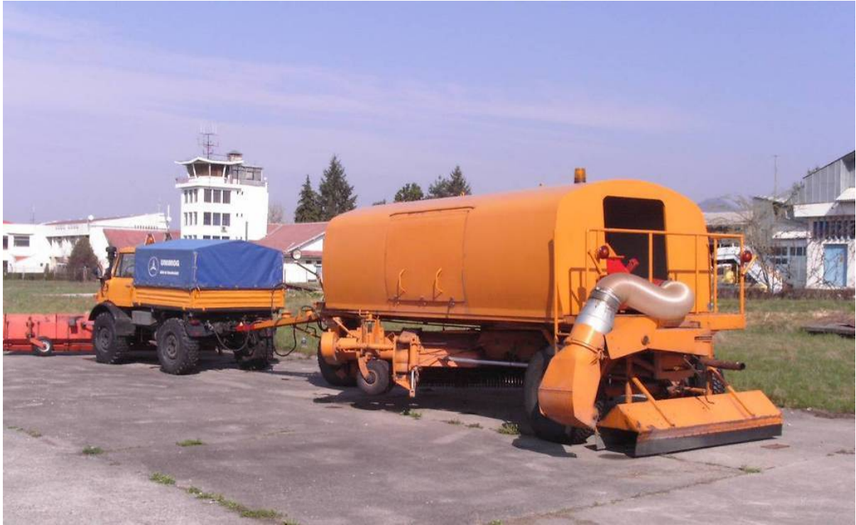
De-icing equipment with the Terminal and ATC Tower in the background
