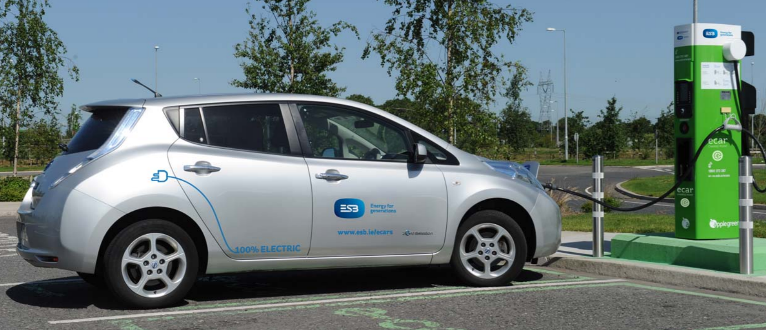
Figure 6 EV Fast Charge Point
