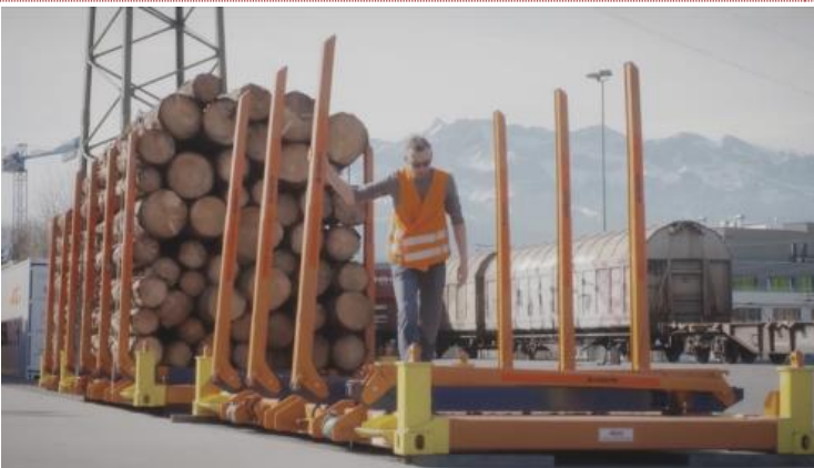
Empty timber cassette folding of stanchions and preparation for stacking
