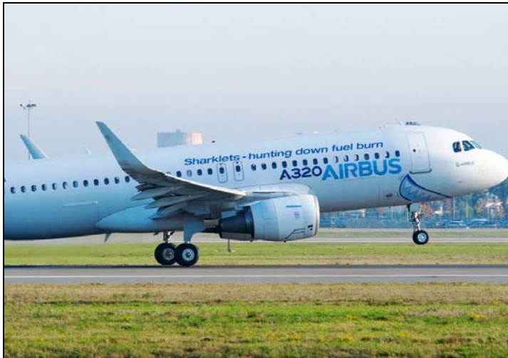
Figure 8.2: A320 with sharklets for fuel burn research - maiden flight from Toulouse - November 2011
