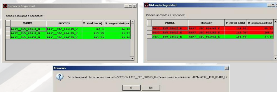
Illustration 55. Warning message after detection of safety distance violation and alarm application interface Source: DGT
