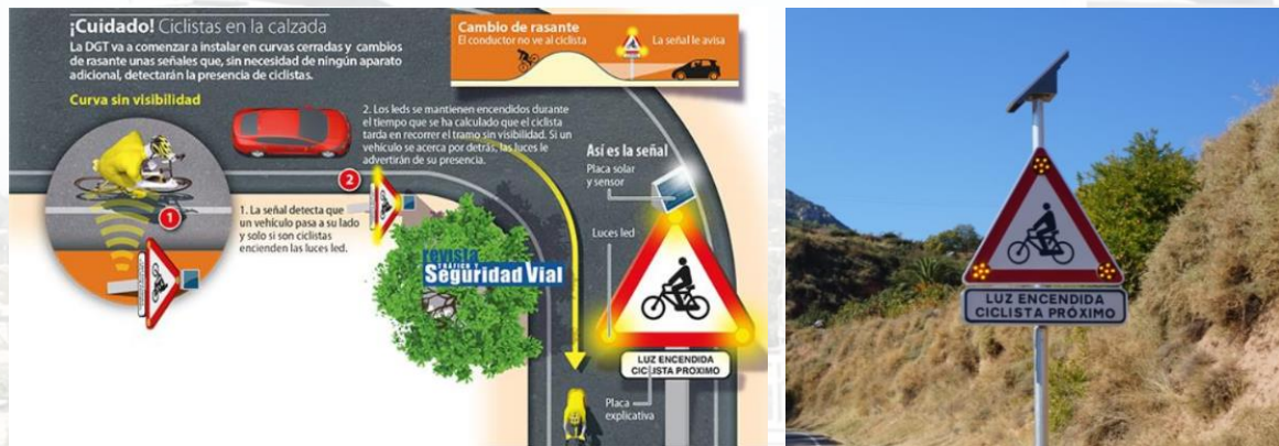
Illustration 51. Functional diagram of the dynamic signalling warning about the presence of cyclists and example of installation. Source: DGT
