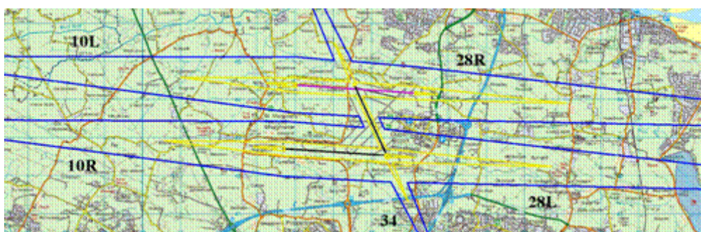
Figure 11. Extract from Fingal County Development Plan 2006-2011. Risk contours for Dublin Airport, including proposed Northern Parallel Runway 10L/28R in the current Fingal County Development Plan.
