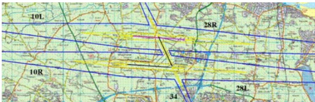
Figure 8. Extract from Fingal County Development Plan 2006-2011. Risk contours for Dublin Airport, including proposed Northern Parallel Runway 10L/28R in the current Fingal County Development Plan.
