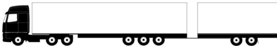
Type 2: Tractor with ordinary semi-trailer and centre axle trailer
