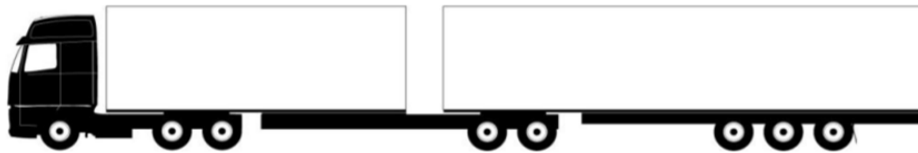
Type 3: Tractor with link trailer and ordinary semi-trailer
