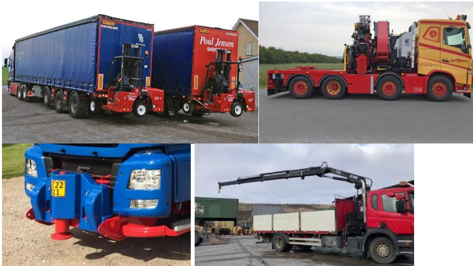
Figure 9. Illustrations of typical vehicles included in the segment (truck mounted forklift, foldable cranes and support legs).
