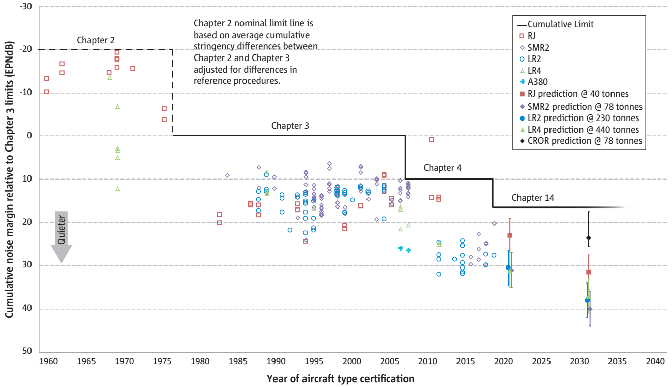
Figure 2.2 Improvement in aircraft noise performance has occurred over time
