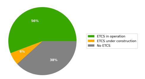
ETCS current status of CNC lengths expected according to TEN-T Guidelines by 2030
