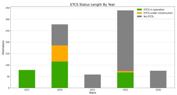
ETCS deployment progress against the EDP targets per year. Note: The 2030 bar includes sections planned in the EDP as "beyond 2023"
