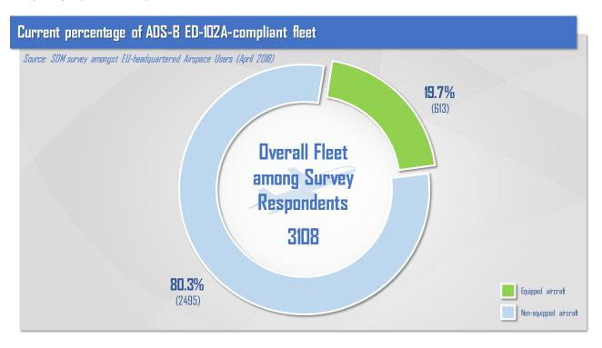
As can be seen only around 20% of the EU operator's fleets are compliant with ED-102A (DO-260B), the majority of these are forward fit on new deliveries, as off the last few years, once it became known that this would be the required standard for the future. It can be assumed that this percentage is a good representation of the overall European fleet equipage rate.
