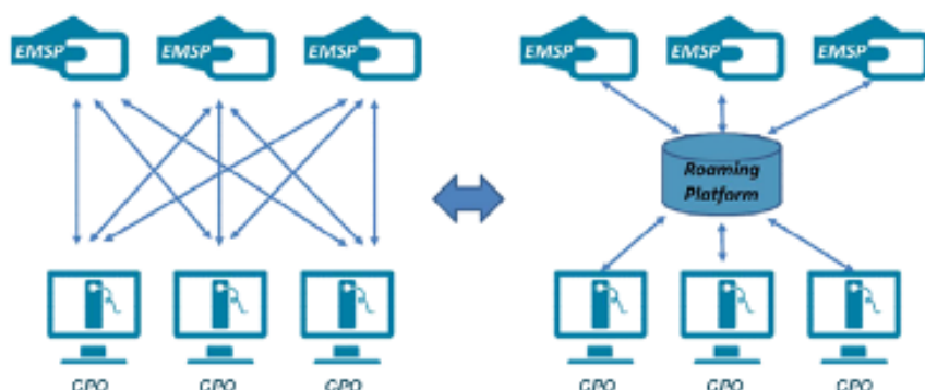
Figure 21: peer-to-peer roaming (left) versus roaming via a platform (right)
