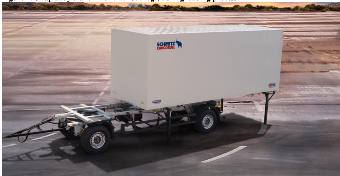
Figure 4: Swap body trailer with extended legs, during loading process.
