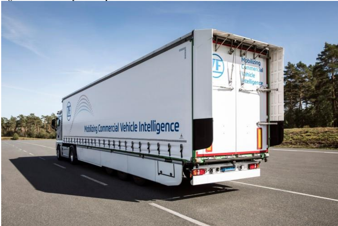
Figure 17: Rear aerodynamic flaps on a semitrailer
