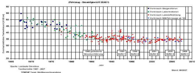
Indeed, as the graph shows, engine efficiency development is offset by stringent NOx emission requirements.
