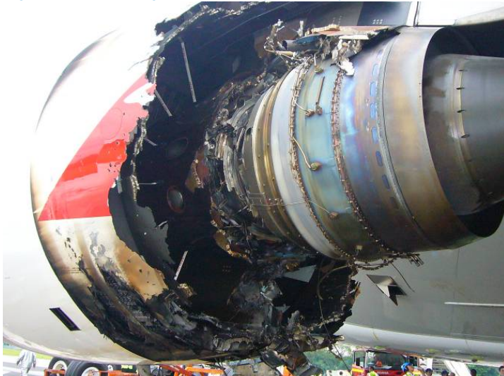
Figure 9.3: Damage Sustained by No 2 engine of A380-842 VH-OQA
