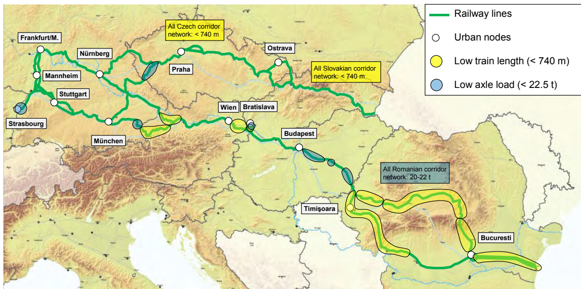
Figure 14: Areas with critical line layout – Train length and axle load
