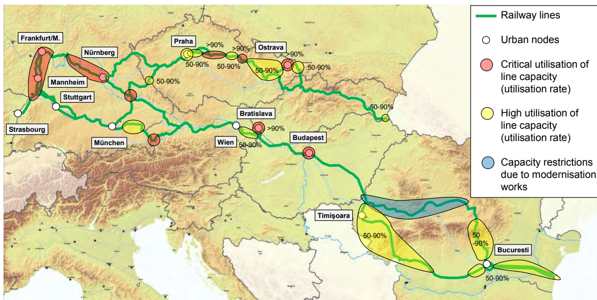
Figure 12: Areas with high rail capacity utilisation on the Rhine-Danube Corridor
