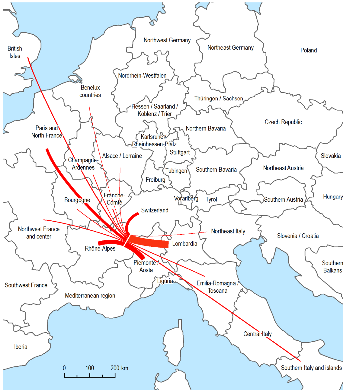
Figure 9: Share of origin and destination regions of freight traffic on the road at Mont Blanc tunnel
