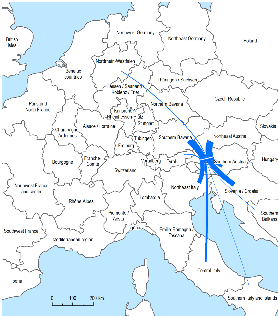
Figure 21: Share of origin and destination regions of freight traffic on rail at Tauern
