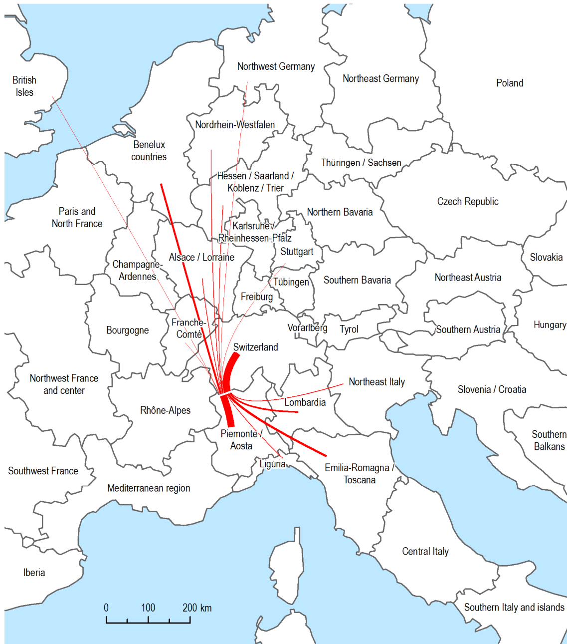
Figure 10: Share of origin and destination regions of freight traffic on the road at Gd St-Bernard
