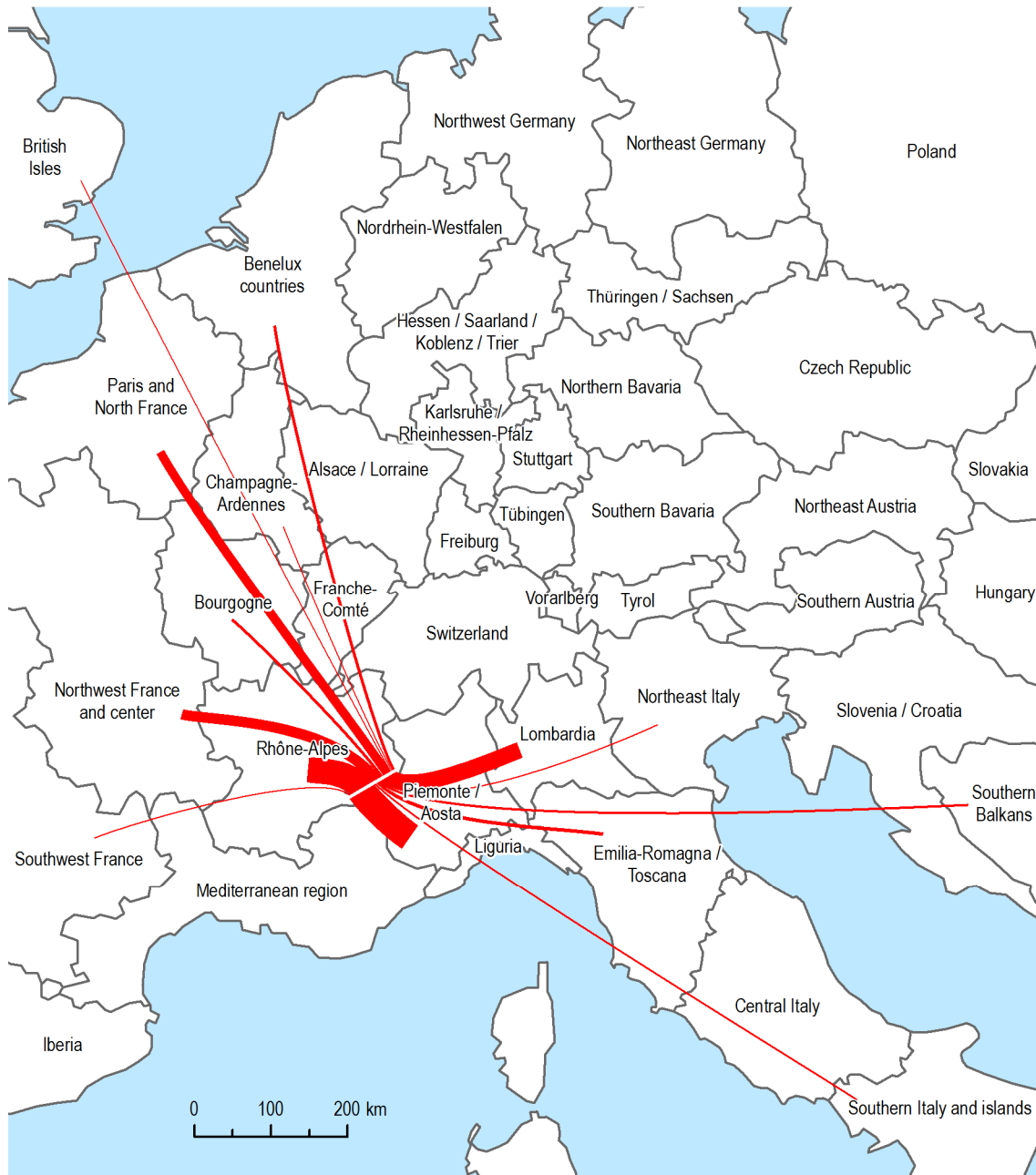
Figure 8: Share of origin and destination regions of freight traffic on the road at Fréjus tunnel
