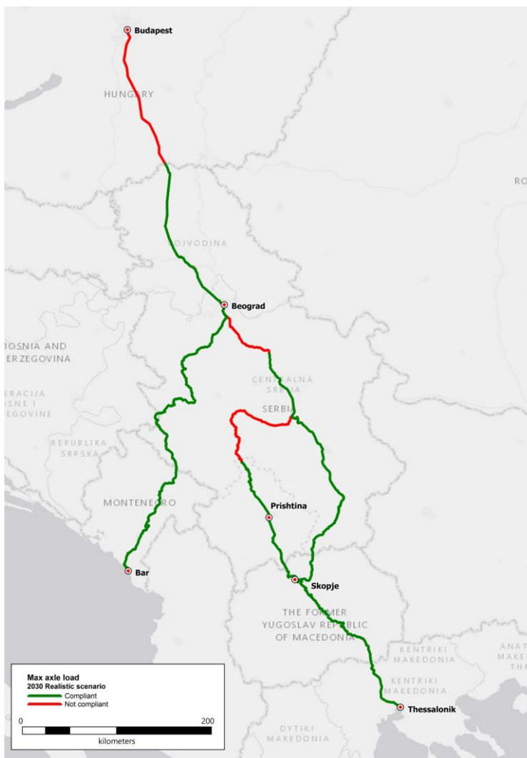
Figure 21: Maximum axle load on the OEM related WB6 corridor - Realistic scenario (2030)
