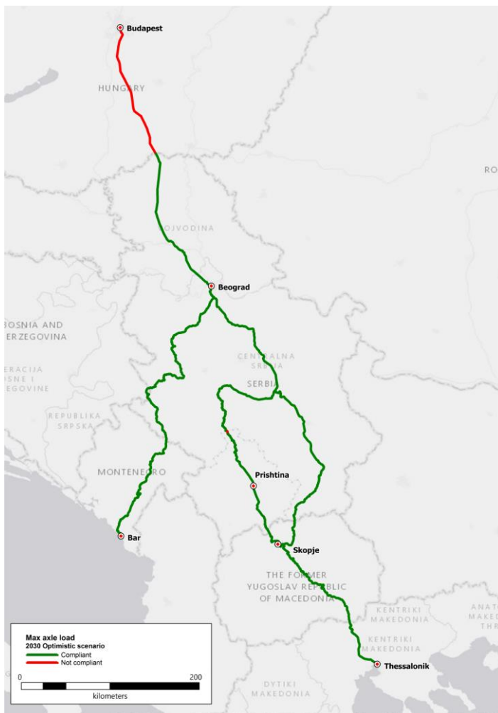
Figure 25: Maximum axle load on the OEM related railway core network in WB6 - Optimistic scenario (2030)
