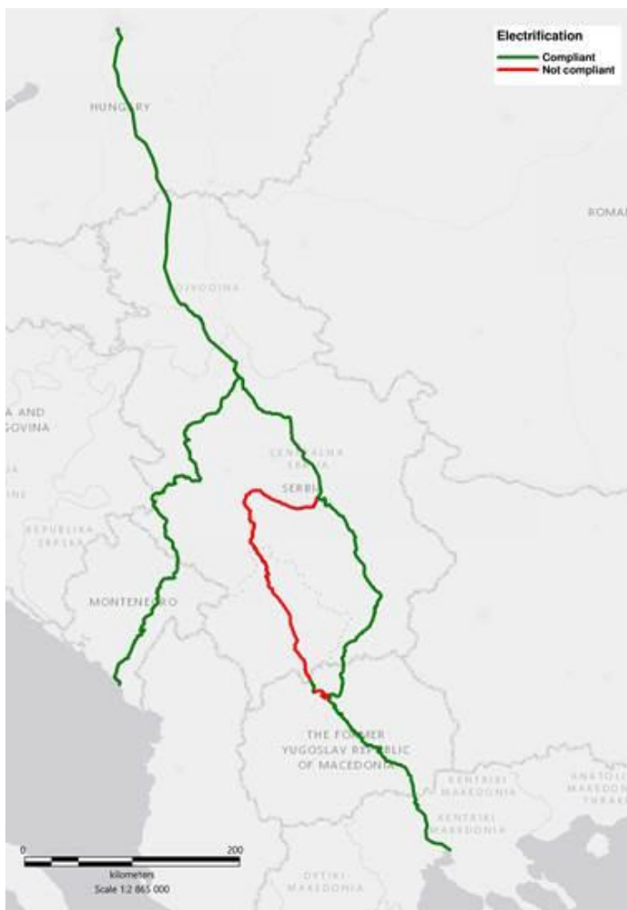
Figure 10: Electrification on the OEM WB rail network
