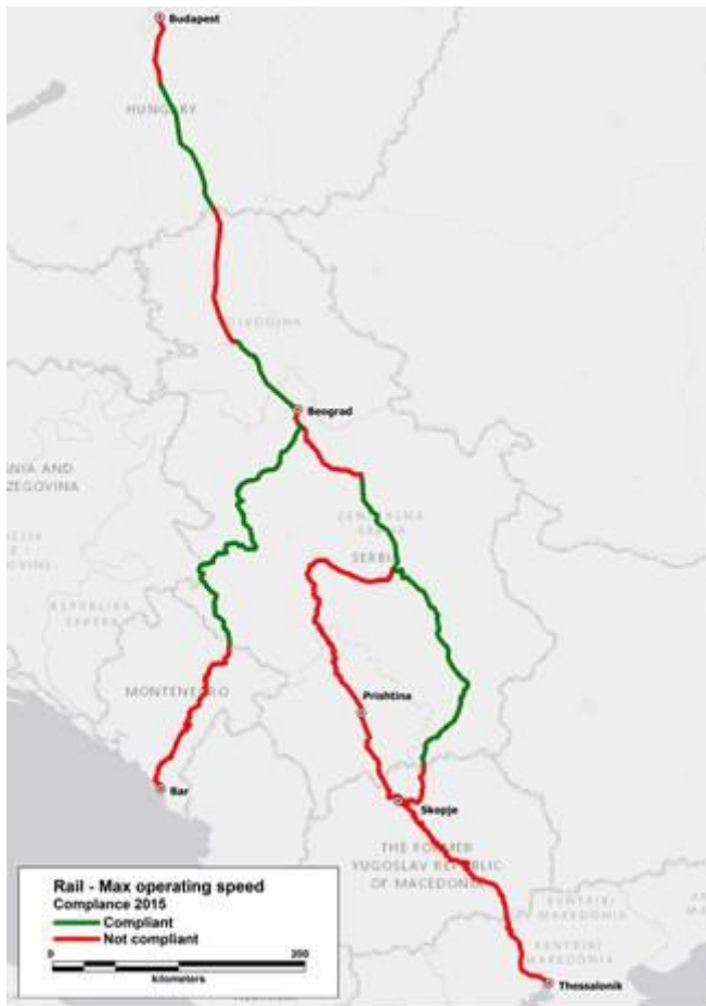
Figure 7: Maximum operating speed on the OEM WB rail network (2014)
