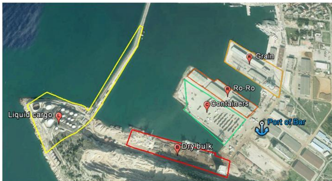
Figure 12: The layout of the Bar port along with its terminals
