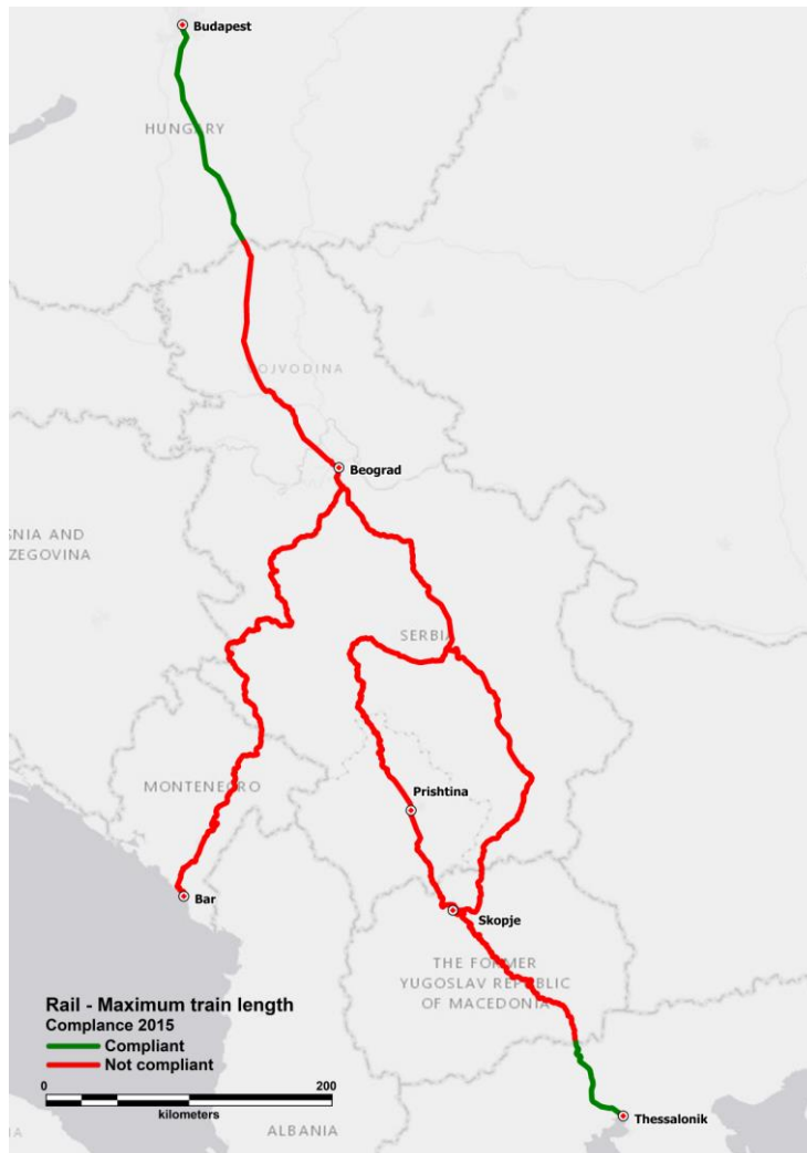
Figure 8: Maximum train length on the OEM WB rail network (2014)
