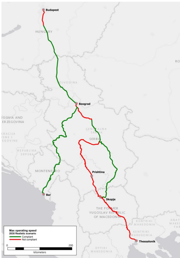
Figure 19: Maximum operating speed on the OEM related railway core network in WB6 - Realistic scenario (2030)
