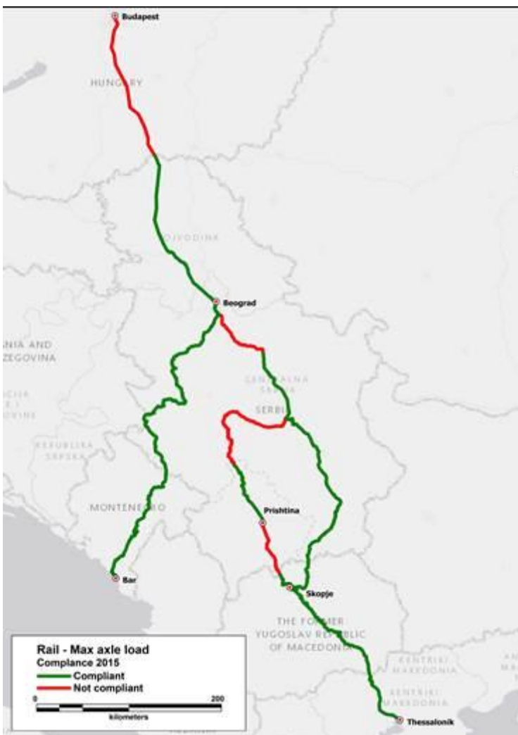
Figure 9: Maximum axle load on the OEM WB rail network
