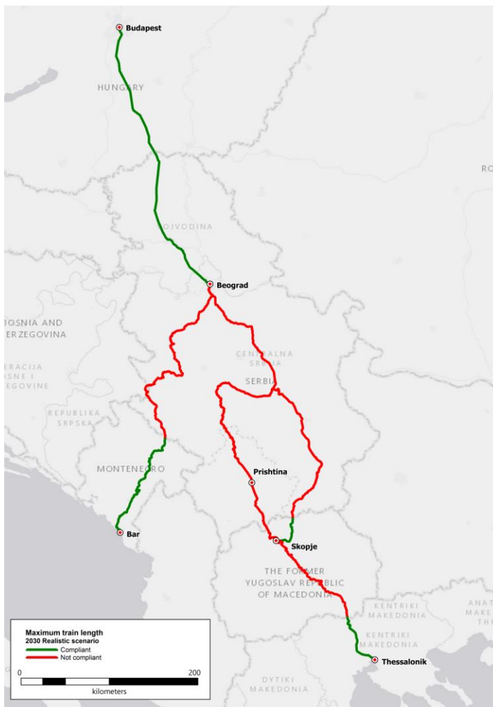
Figure 20: Train length on the OEM related railway core network in WB6 - Realistic scenario (2030)
