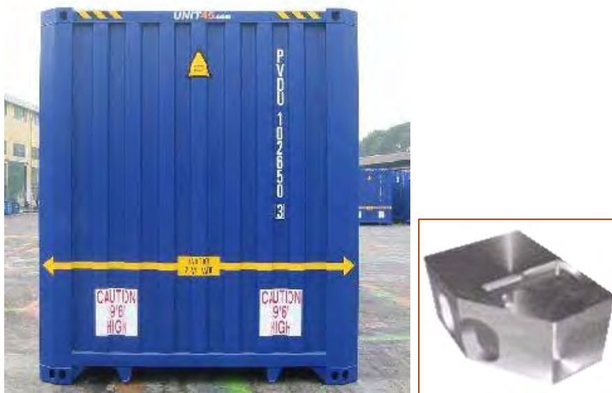
Figure 4: 45’ long domestic European container with special corner casting
