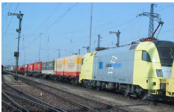
Unaccompanied CT service carrying swap bodies and piggyback trailers, without road vehicle tractor units or drivers Unaccompanied CT service carrying maritime containers
