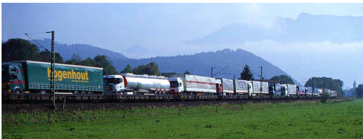
Accompanied CT service carrying entire lorries, with lorry drivers travelling in a passenger coach (at the far right-hand end of the train immediately behind the locomotive)
