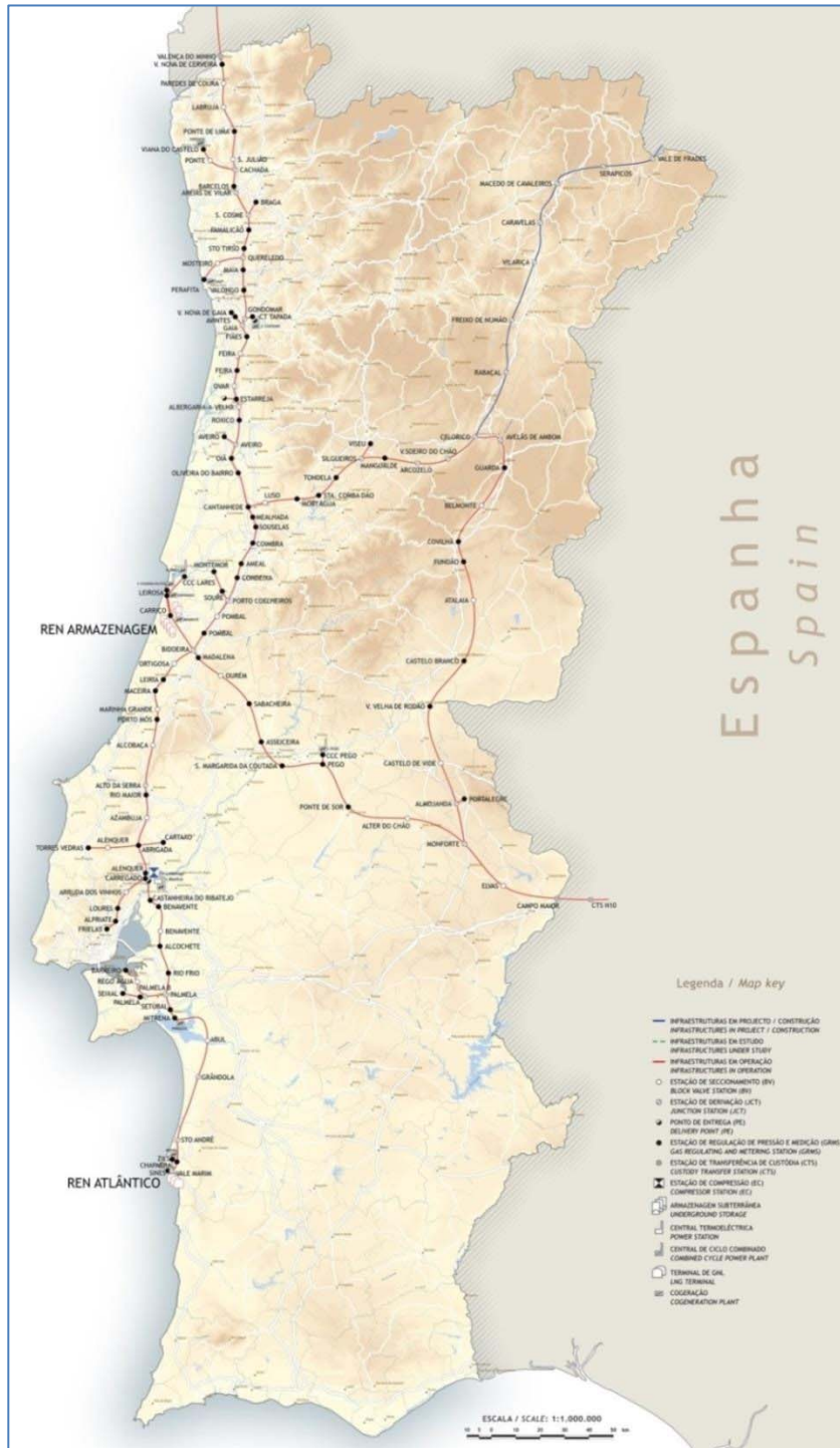
Figure 22 - National Natural Gas Transmission Network. Source: REN.
