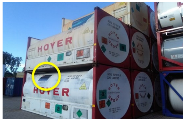
Figure 23 - One of the two tracking devices installed on board of one of the two tank containers
