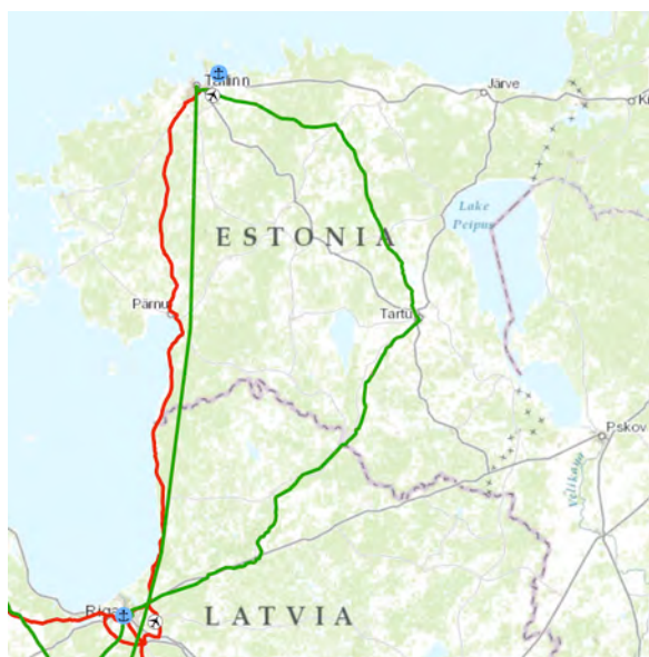
Figure: The existing 1520 mm gauge railway infrastructure shows in the map as green line via Tartu in eastern Estonia. The planned 1435 mm European standard gauge railway would run south from Tallinn the shortest way to the Latvian border (green line) in parallel to Via Baltica. (TENtec)
