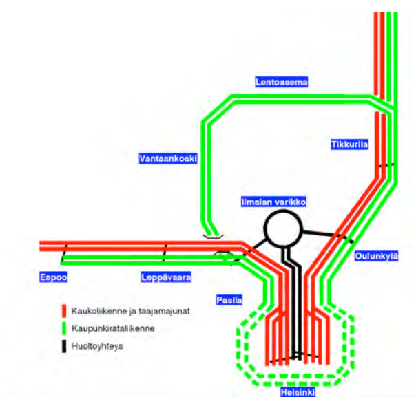
Figure: The transport model of the Helsinki urban node that consists of the main railway (red) and urban train connections (green). Ring Rail will connect (in 2015) Helsinki Airport to the main railway (red) and city centre by urban rail. City Rail Loop will extend the urban railway around the city centre (estim. 2026). This will allow trains to go across the Helsinki urban node, while currently the city centre is a railway end station. The urban train network will also be connected to the metro system (not shown in the figure). The Espoo city rail project will be completed by 2025 (estimation). (Source Finnish Transport Agency)
