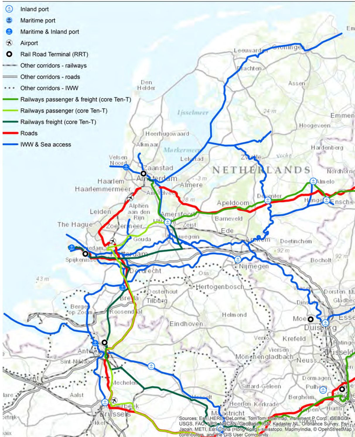
Figure 1: Alignment of sections (Road, Rail and IWW) and nodes (maritime port, inland port, airport, RRT) in the Netherlands along the North Sea – Baltic Corridor as well as the alignment of sections of other CNC traversing the Netherlands
