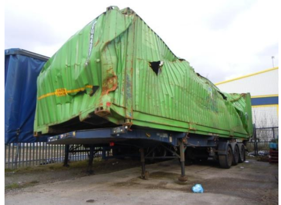
Figure 7.1: Container Trailer following an incident showing severe damage to the box
