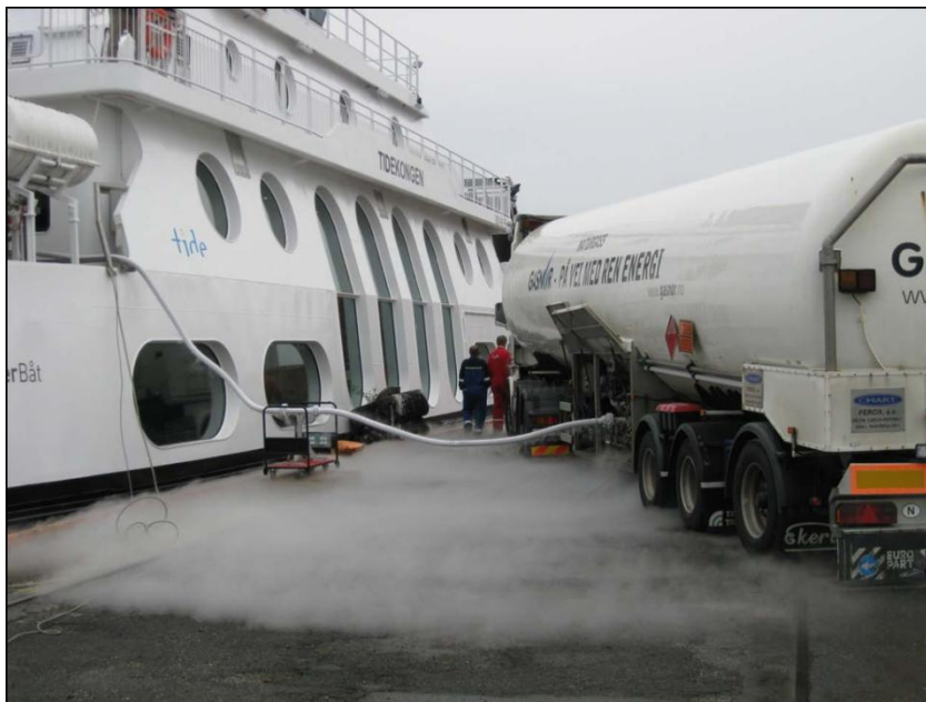
Figure 8.1: LNG Refuelling using a Tank Truck
