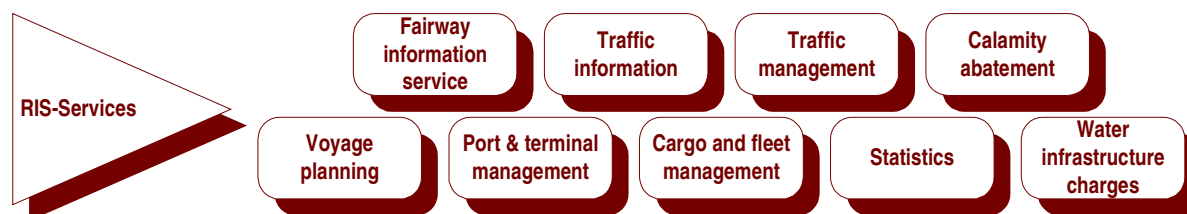
Figure 30. RIS – main services Source: PIANC, 2001
