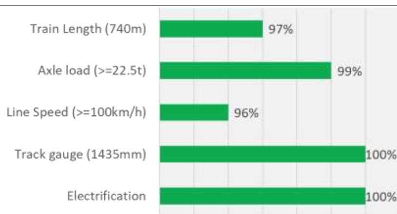
Figure 2-3: NSMED Rail compliance with TEN-T regulations, status December 2022
