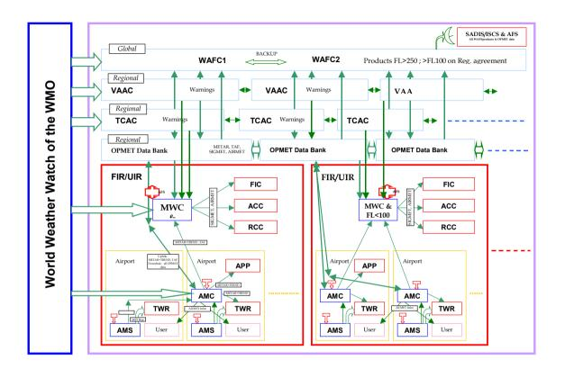
Legend: — Meteorological information circulation - \_\_\_\_ air navigation structures - \_\_\_\_ meteorological structures - \_\_\_\_ meteorological structures - \_\_\_\_ : AFS and/or GTS reception - \_\_\_\_ : AFS/GTS mission and reception
