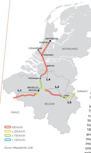
HSL Zuid is a 125 km-long high-speed rail line that runs between the Netherlands and the Belgian border. Together with the Belgian HSL 4 line, HSL Zuid connects Schiphol via Rotterdam to Brussels and Paris (part of the PBKAL – Paris-Brussels-Koln-Amsterdam-London – corridor). Operations between Rotterdam and Amsterdam with ETCS Level 1 started in September 2009. This section of the line will switch to ETCS Level 2 (L2) in mid-2010.
