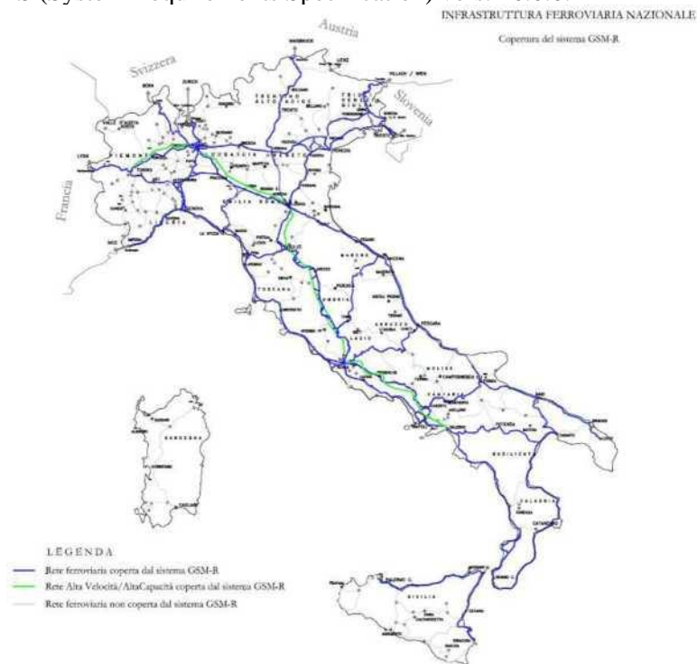
Figure title: Italy’s Railway Infrastructure – GSM-R system coverage
