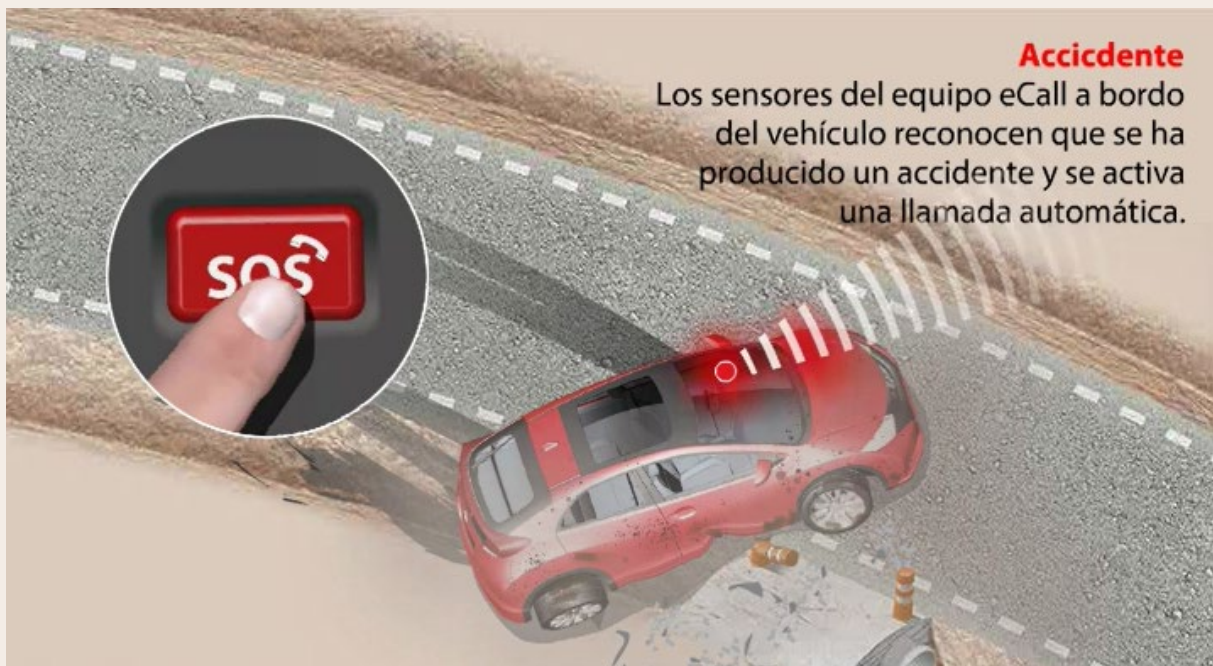
Illustration 79. How eCall Works in Spain. Source: DGT Magazine
