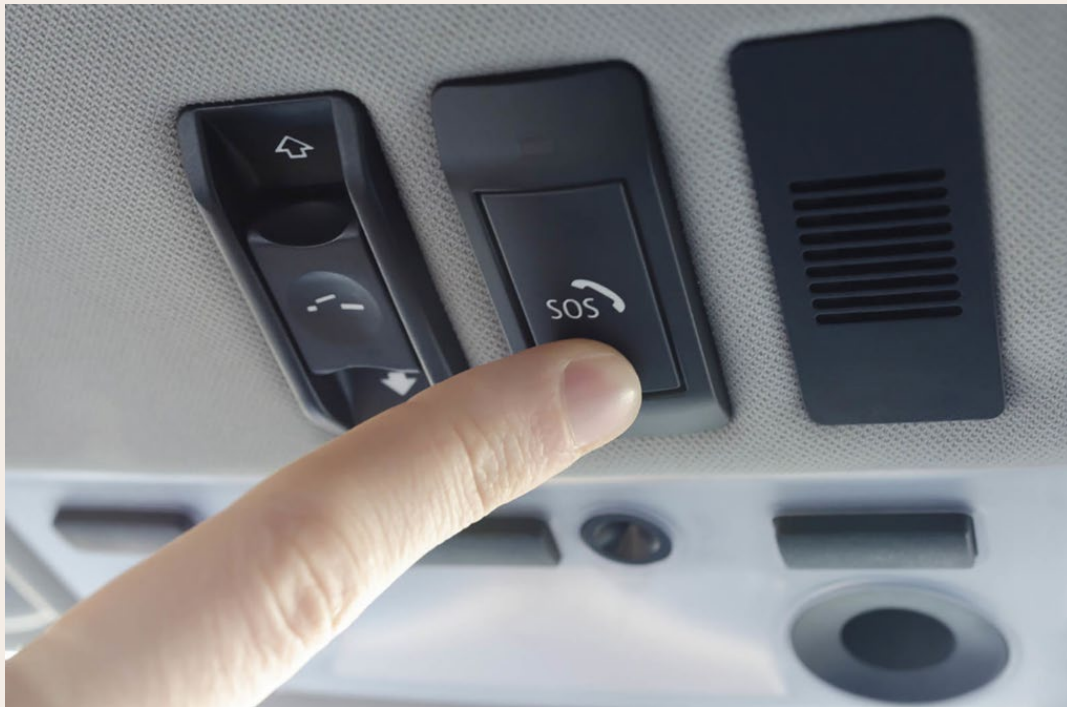
Illustration 78. eCall – The lifebutton. Source: DGT Magazine
