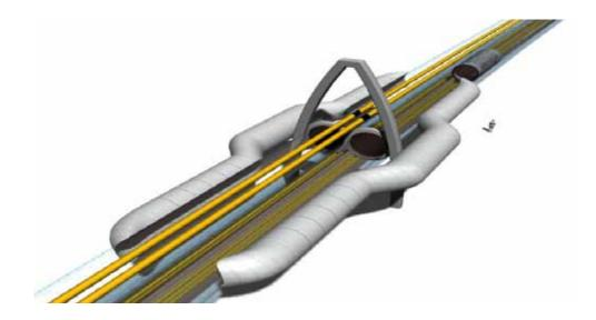
Distribution locks are placed before and after stations as wells as at feeders and branching-off points which are shut by sliding doors. A branching-off point is a chamfer bifurcation with a double lock. By shutting off one of the pipes, the cabins follow the directional suction of the open track. Feeders work after the zipper mode by regulating the amount of air as in the stations described afore.
