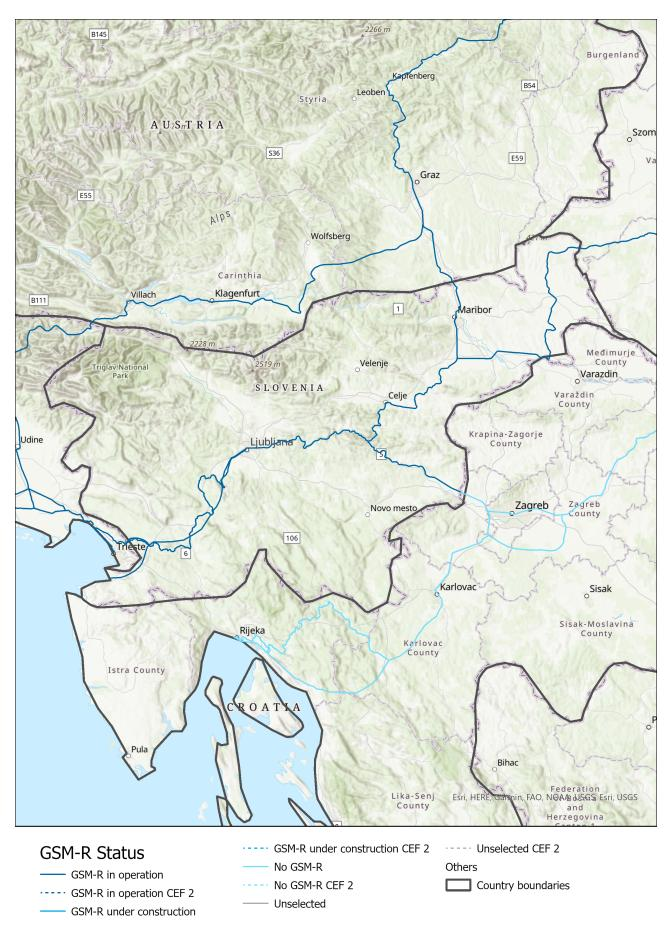
Overview of the GSM-R deployment (Source: DMT elaboration)
