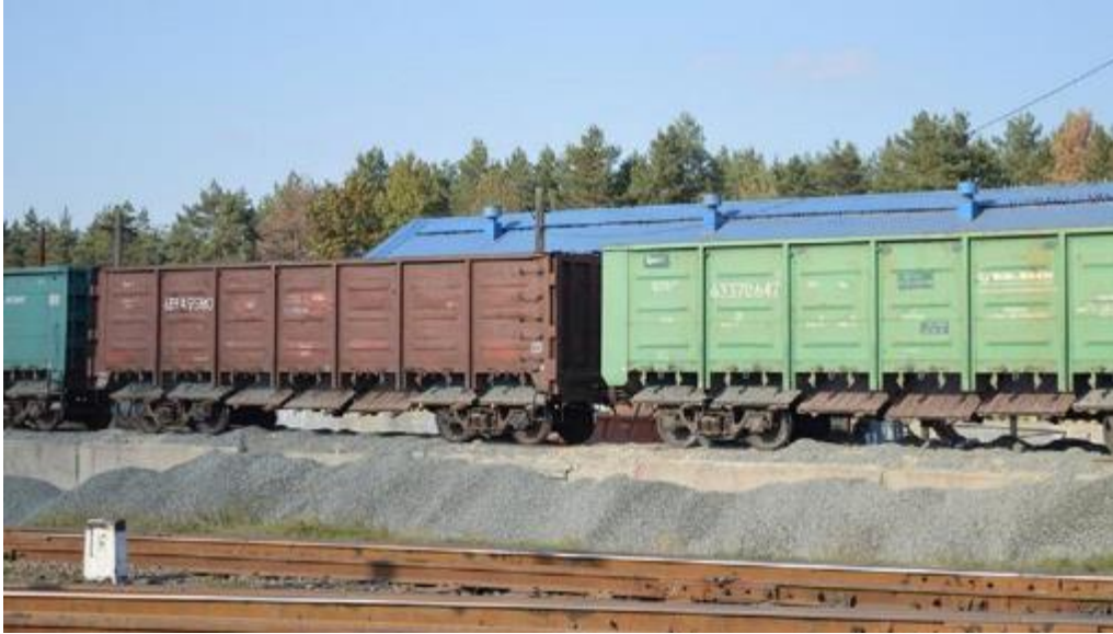
Figure 4.3: Open box or “gondola” wagons. Source: prepared for JASPERS by Egis
