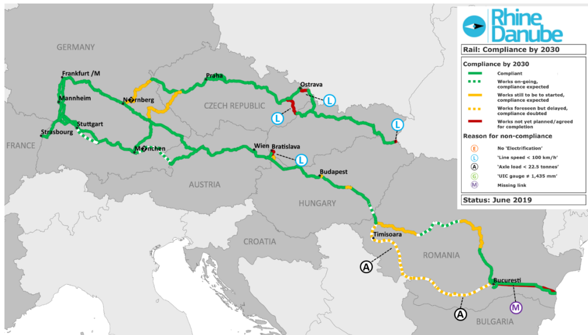
Figure 3: Rail compliance by 2030 overview
