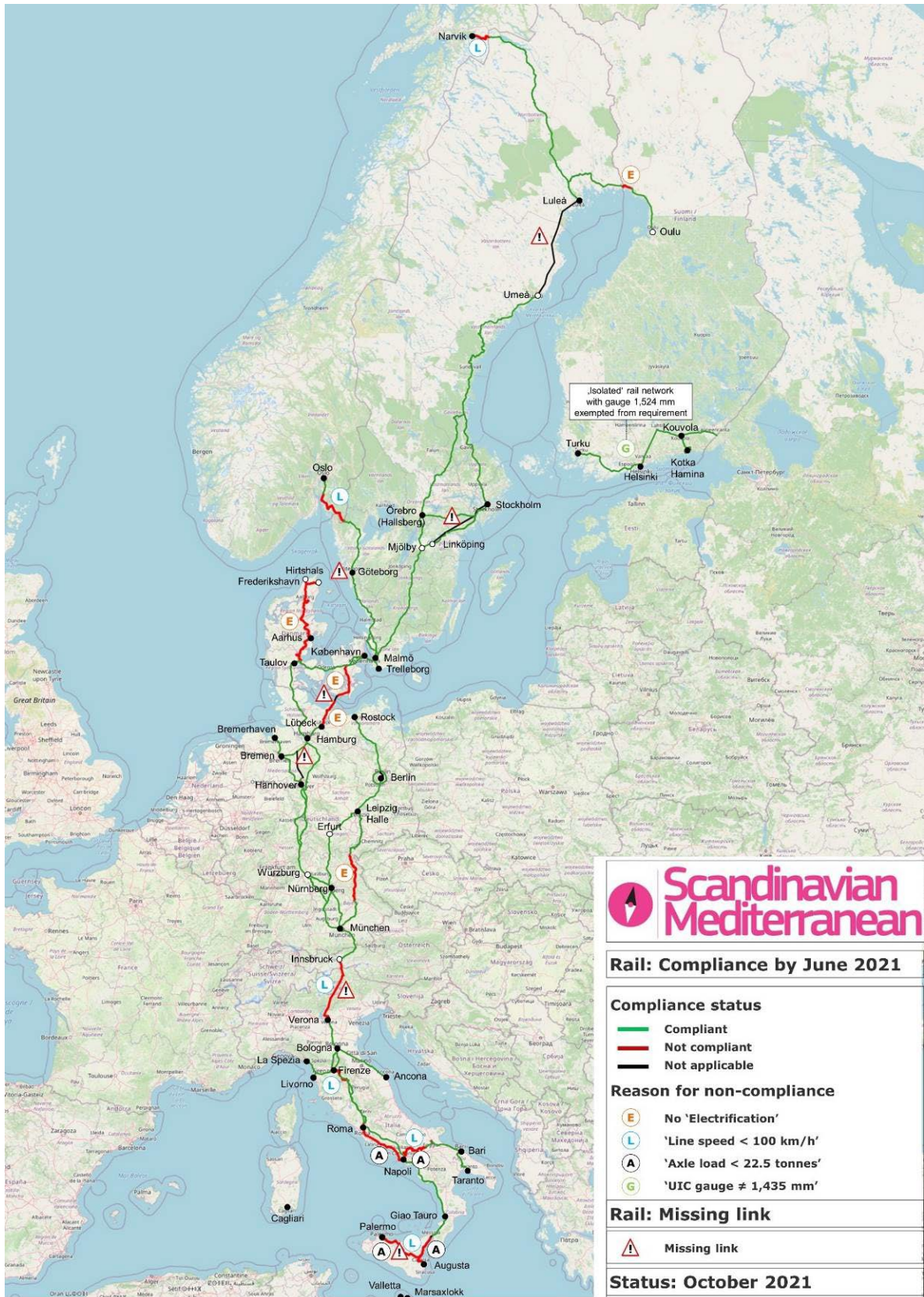
Figure 2: Rail compliance by June 2021 for KPIs 'Electrification', 'Line speed', 'Axle load', and 'Track gauge' and for 'Missing links'
