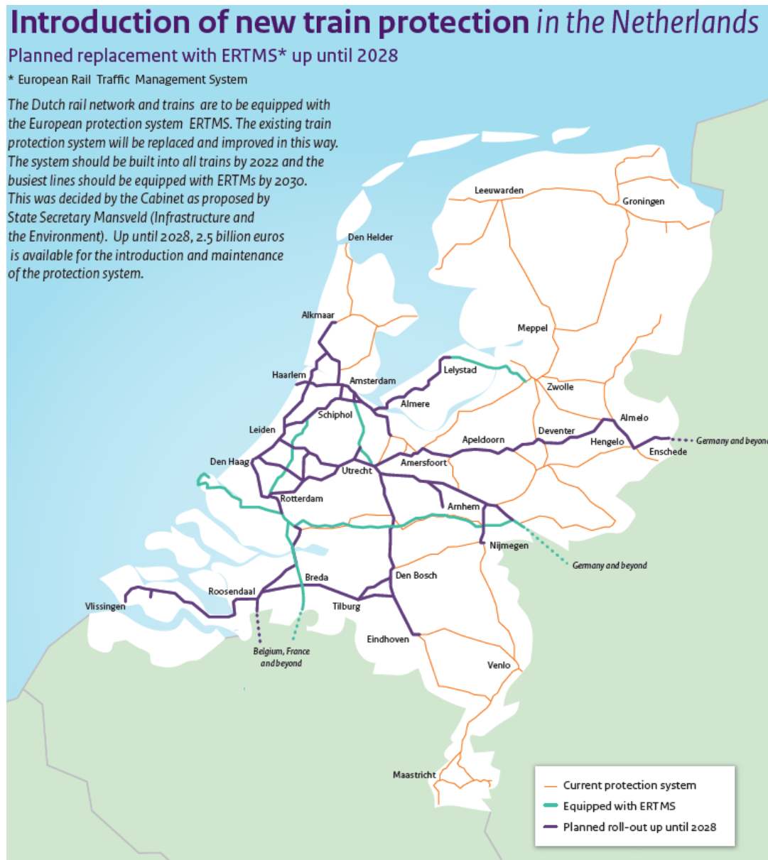
Figure 86 : Introduction of ERTMS in the Netherlands
