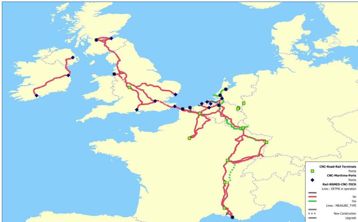
Figure 31: ERTMS Deployment on NSMED corridor
