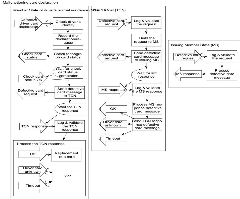
Figure 4 – “Malfunctioning card declaration” process
