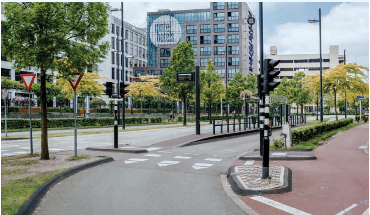
Figure 10: Separated traffic flows. Cycling path is parallel to the bus lane and cyclists have priority over the car traffic. (Picture: Shutterstock, 2016)
