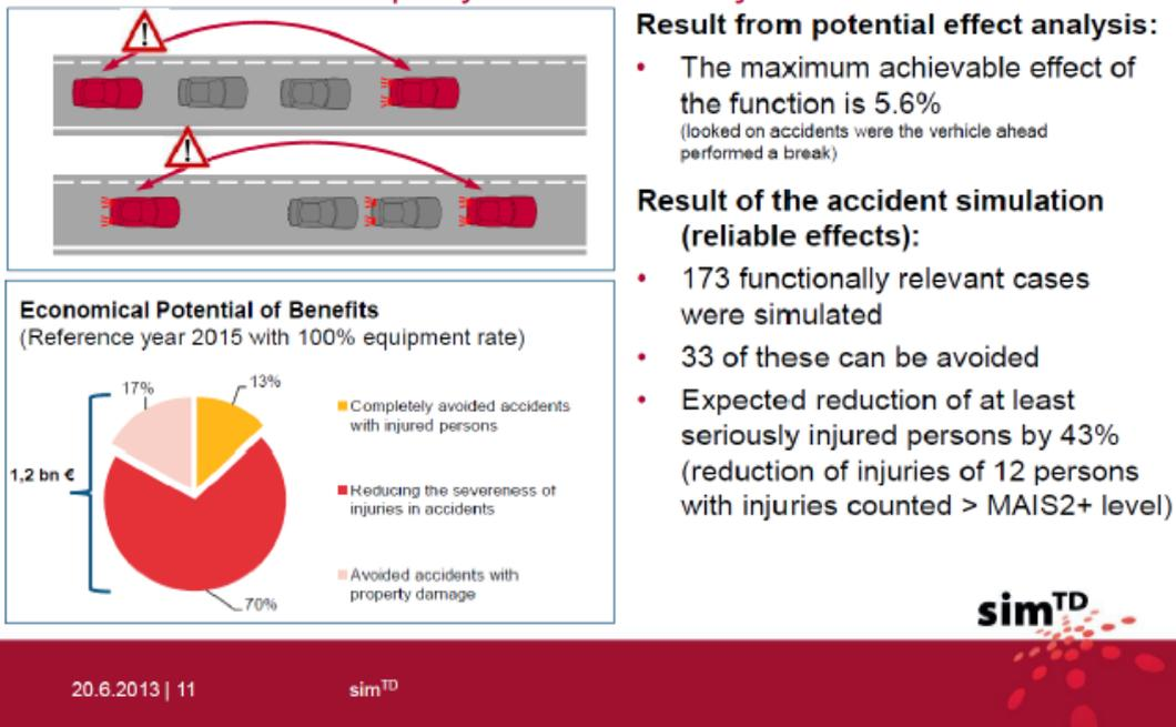
Figure 9 – Reliable effect of Electronic Brake Light (ITS-G5)
